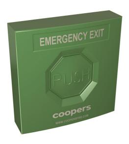
The standard emergency retract button is a simple solution made of polycarbonate / ABS plastic. This system is vandal resistant and can be used with standard recessed simple gang back box. simply press the button and the curtain will raise for a predetermined amount of time, after this time it will lower sealing the opening.
