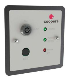
The Zone Control Panel Remote (ZCP-R) is an optional test station that can be used with the BBU (Battery BackUp Unit) and ERU (Emergency Retract Unit) systems. The ZCP-R provides LED indication of the status of the power supply and of the alarm. The ZCP-R also includes a key switch and reset button for localised testing of the associated curtain(s) controlled by the BBU / ERU.
