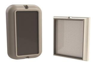
The Obstruction Warning System monitors the opening protected by a fire curtain to ensure the opening is kept clear. If the opening is obstructed then the infrared beam is broken. After a short delay a warning device will be activated.
