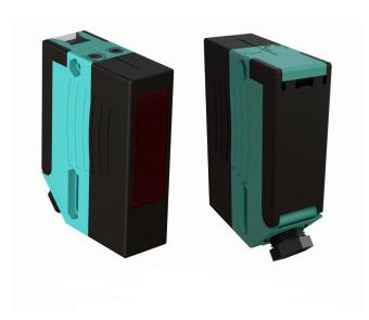
The Obstruction Warning System monitors the horizontal opening protected by a fire curtain to ensure it is kept clear. If the opening is obstructed the LED beam will be broken. After a short delay period a warning device will be activated. The warning device can be audible and/or visual.
