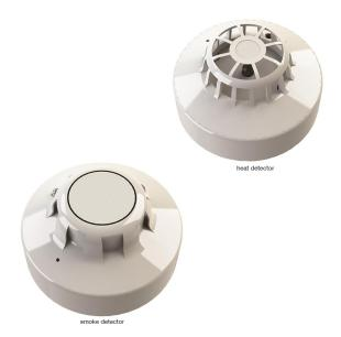
The Series 65 Optical Smoke Detector (OSD) and heat detector (HD) has a moulded self-extinguishing white polycarbonate case. The OSD chamber houses an infrared light emitting diode (LED) and a photo-diode. If light is scattered onto the photo-diode due to the presence of smoke – the detector switches the alarm on. The HD monitors air temperature electronically and is initiated if the ratio exceeds the factory pre-set level.
