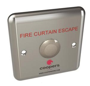
Our stainless steel egress button, is used to operate a curtain once it is deployed. This allows egress after deployment ensuring safe escape. simply press the button and the curtain will raise for a predetermined amount of time, after this time it will lower sealing the opening.
