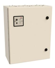
The Variospeed®6 BBU-CG system is used for Smoke / Fire Curtain(s) fitted with 24Vdc permanent magnet electrical motors fitted with an internal 24Vdc electromagnetic brake, as standard. When the Smoke / Fire curtain(s) are fully retracted, the internal electromagnetic brake is powered, keeping the Smoke / Fire curtain(s) in their retracted position.
