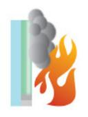
The filler interlayer begins to form an opaque insulating protective layer resisting further penetration.
