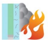
Initially the fire causes the glass pane that is towards the fire side to break due to the stress on the glass.
