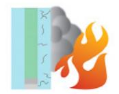
Initially the fire causes the glass pane that is towards the fire side to break due to the stress on the glass.
