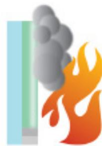
The filler interlayer begins to form an opaque insulating protective layer resisting further penetration.
