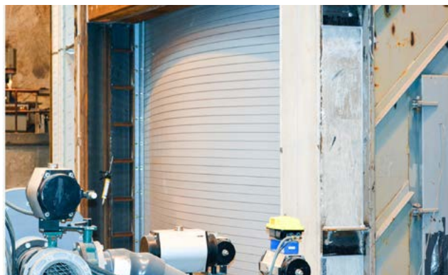
The SafeSpace 500 was subjected to both positive and negative pressure equal to 1.2 times the 255 mph (410 kph) design wind load
