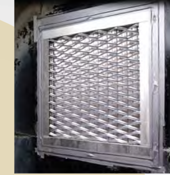
A test panel of INNIVATE VITAL Series Performance Louvre undergoing testing to BS EN 13030:2001
