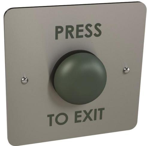
This is an easy to use emergency egress button which is fixed on a stainless steel plate. It can be used with standard recessed single gang box or surface mounted. simply press the button and the curtain will raise for a predetermined amount of time, after this time it will lower sealing the opening.
