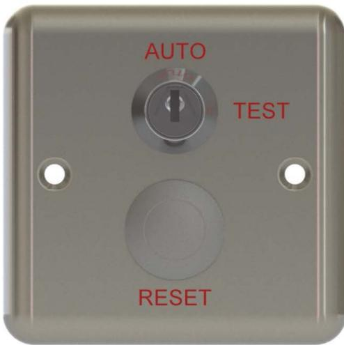
The Test Reset Switch (TRS) can be used with all Battery Back-Up Unit (BBU) and Emergency Retract Unit (ERU) . It is a robust alternative to the ZCP-R and provides a key switch and reset button for localised testing of the associated curtain(s) controlled by the BBU / ERU. The TRS can be flush or surface mounted and Multiple TRS can be used with each BBU / ERU.
