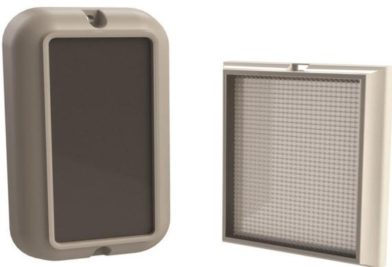
The Obstruction Warning System monitors the opening protected by a fire curtain to ensure the opening is kept clear. If the opening is obstructed then the infrared beam is broken. After a short delay a warning device will be activated.
