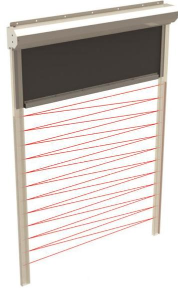
The Obstruction Light Curtain monitors the opening protected by a fire curtain to ensure the opening is kept clear. If the opening is obstructed then the infrared beam is broken. After a delay a warning device will be activated.
