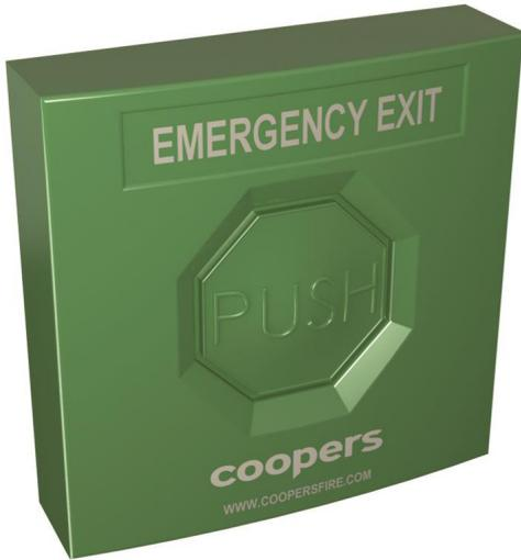
The standard emergency retract button is a simple solution made of polycarbonate / ABS plastic. This system is vandal resistant and can be used with standard recessed simple gang back box. simply press the button and the curtain will raise for a predetermined amount of time, after this time it will lower sealing the opening.
