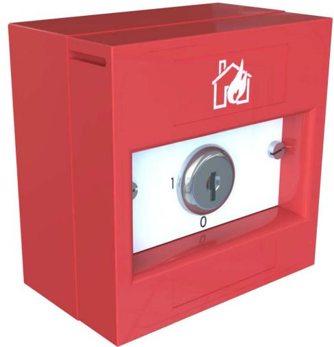
The Coopers Fire Standard Key Switch can be used on Variospeed®6 or MK5 control systems. It can be used as a remote means of testing the Fire/Smoke curtains. The Standard Key Switch can also be used to reset stand-alone smoke/heat detectors when connected to the Variospeed®6 control system.
